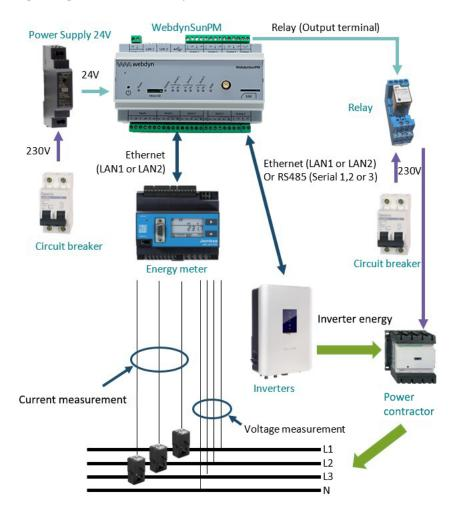
This wiring must use the following elements or equivalent and be adapted to your solar installation including a WebdynSunPM:
