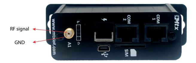
These external antennas must be matched properly to achieve the best performance regarding radiated power, DC-power consumption, modulation accuracy and harmonic suppression.
