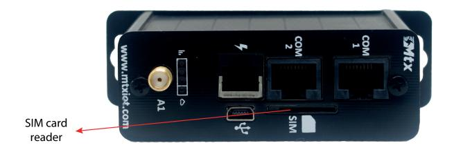
The card holder is a five wire interface according to GSM 11.11. It has a SIM card detector switch to detect whether or not the SIM card drawer is inserted.
