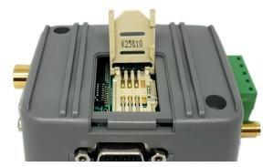
The card holder is a five wire interface according to GSM 11.11. It has a SIM card detector switch to detect whether or not the SIM card drawer is inserted.
