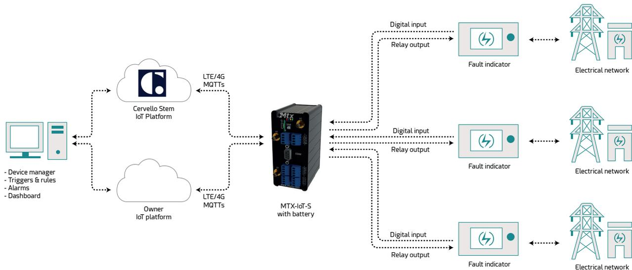
In these cases, the maintenance manager needs to know in real time, the status of each of the critical points. To do this, several fault indicators are used. These devices contain an internal relay that opens when the sensor detects ground faults or short circuits. In case of detection, the internal relay opens and sends a digital fault signal. Once the fault has been signaled, an external relay is required to reset the device to return to the initial monitoring point.
