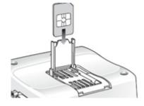
The card holder is a five wire interface according to GSM 11.11. It has a SIM card detector switch to detect whether or not the SIM card drawer is inserted.
