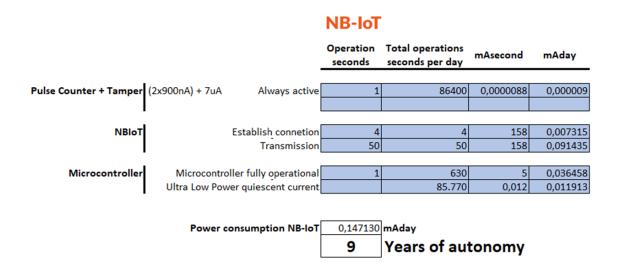
Applying the annual self-discharge coefficient gives us a result of an estimated life span of the batteries of 9 years.
