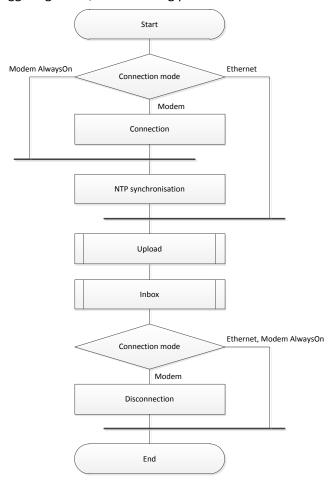
In case of failure of the GPRS data connection, a new connection will be tried one hour later unless a new connection was initiated in the meantime (by explicit request, or triggered by an alarm or by a periodic upload). This is illustrated below including the delayed disconnection.
