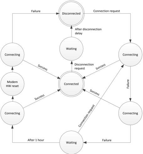
If 10 iterations of the loop "Connecting -> Connecting -> Waiting" (the 3 states on the bottom right) is detected, the transition to the next state is forced without waiting 1 hour.
