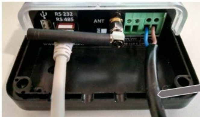
Enclosure opening for Mains Power Supply cable
