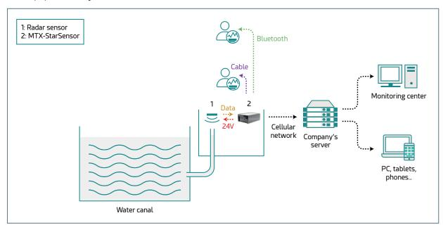
Webdyn's MTX-StarSensor is an autonomous modem that powers any radar sensor to measure the water level of the canals, without the need of a power source, giving the device an autonomy of up to 10 years in case of one daily measurement reading.
