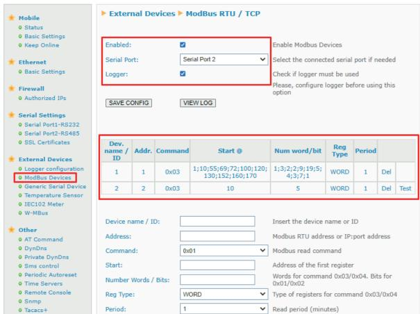
We want to read registers 10,11,12,13,14 from PLC 2. All we need to do is enter register 10 in the "Start" field and 5 in the "Number Words" field (as we want to read 5 registers, from 10 to 14).
