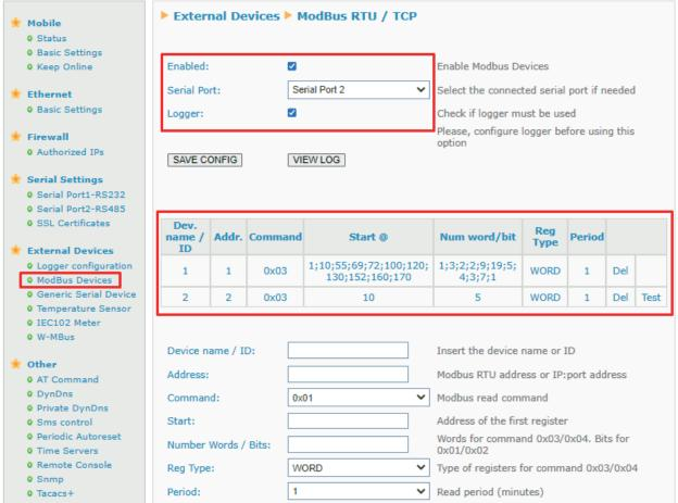
We want to read registers 10,11,12,13,14 from PLC 2. All we need to do is enter register 10 in the "Start" field and 5 in the "Number Words" field (as we want to read 5 registers, from 10 to 14). PLC1 is more complex, since we have a non-consecutive register map. The different blocks of registers we need to read will therefore be separated by ";" (semicolons). This means if we want to read registers:
