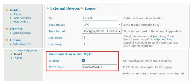
In this screen we have activated MQTT send mode. All data collected by the TITAN-based device will be published in the [IMEI]/logger topic. That the device will replace the [IMEI] tag with your real IMEI. This means that, if the device's IMEI is 357299070082380 (the IMEI can be found in the Mobile > Status menu), the topic used by the TITAN-based device to publish the collected Modbus data will be: 357299070082380/logger.
