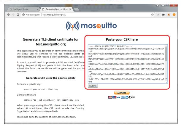
Having generated the client.key and client.crt files, we can insert them at the bottom of the Other > Mqtt page in the TITAN-based device.
