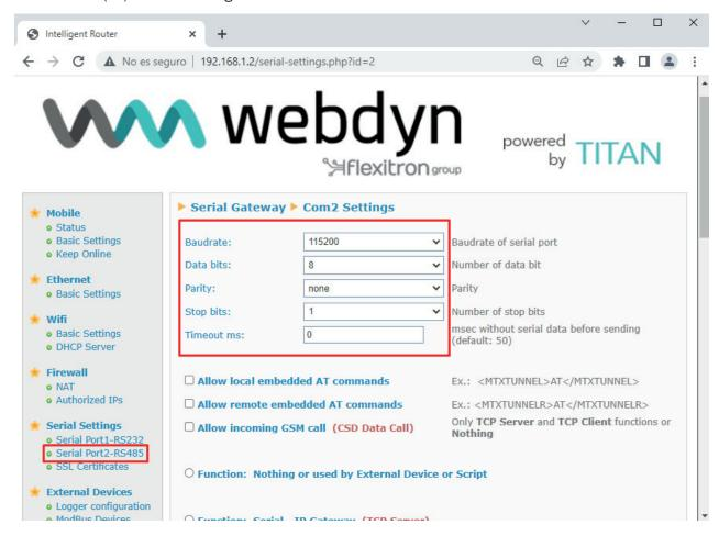
For example, the configuration for the topics of all the serial ports could be as follows:
