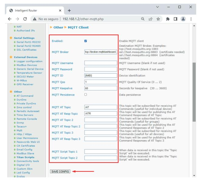
Check with your MQTT broker for the appropriate parameters in this section. Once configured, click on the "SAVE CONFIG" button.
