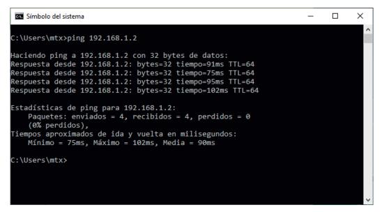
A Ping sent from the PC1 to the PLC via the IPSec VPN:
