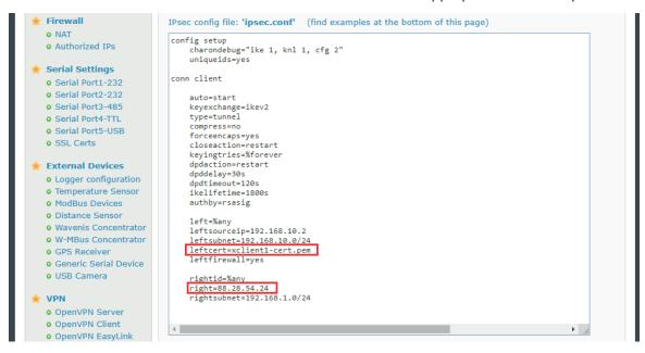
Remember that in "right" you must indicate the public IP of the TITAN-based device acting as the IPSec Master, in this example it is 88.28.54.84. We must also note that the value in leftcert must be "xclient1-cert.pem" in the 2 titans acting as IPSec clients, since this is the name with which the TITAN-based device internally stores the certificate, as can be seen above and as shown in the following image.
