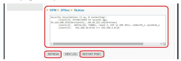
At this point, PLC1 (client) and PLC3 (server) can already interact with each other through a secure IPSec tunnel. Repeat the same procedure for the TITAN-based device connected to PLC2.
