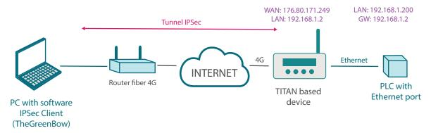
Basically, in this example we want to create an IPSec VPN from a PC (which has an IPSec Client such as TheGreenBow, which is used in this example) to a remote 4G TITAN-based device that will act as an IPSec Server, which in turn has a PLC connected to its Ethernet port.
