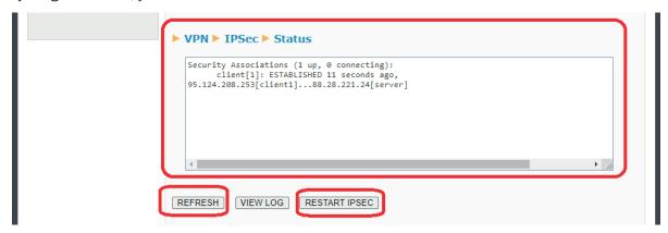
At this point, PLC1 (client) and PLC3 (server) can already interact with each other through a secure IPSec tunnel. For example, you could PING PLC3 from PLC1 and vice versa. Repeat the same configuration procedure for the TITAN-based device connected to PLC2.
