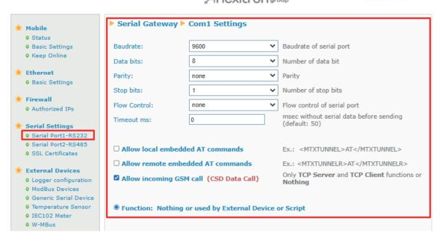
Do the same for the other RS485 serial port in the "Serial Settings > Serial Port2-RS485" menu, configure the screen as follows:
