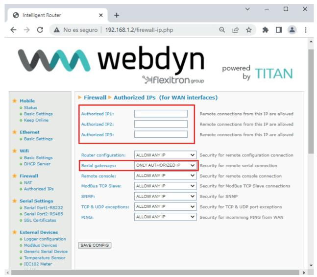
• In this example, 4G/3G/2G to RS232/RS485 gateways have been configured, but TITAN-based devices can be used to configure Ethernet – RS232/RS485 and Wi-Fi – RS232/RS485 gateways in the same way.
