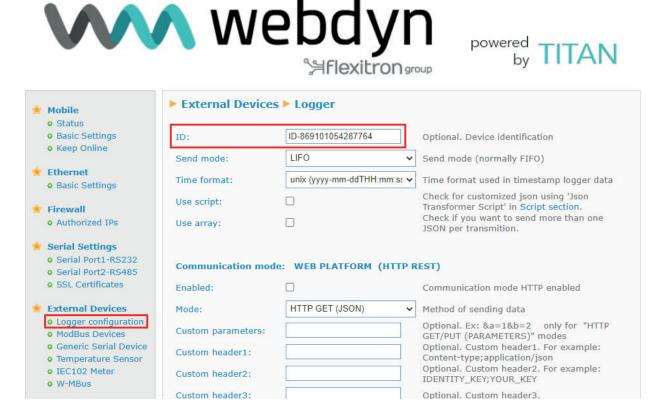
Also in the LOGGER configuration section, at the bottom of the page, the "Enabled" box must be checked to activate the MQTT delivery mode. The delivery topic (the MQTT topic to which the TITAN-based device will send the data) must be set to "/LOGGER" in this example.
