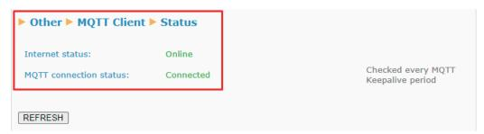
It can also check that the connection exists in the MQTT broker and is well established, by sending an AT command to the TITAN-based device via MQTT. As such, we must configure the /ATR (to receive responses from the executed AT commands) and /LOGGER topics to which the TITAN-based device will send the data read from the Electricity Meter.
