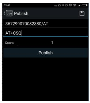
Clicking on the "Publish" button, the command will be received by the TITAN-based device and executed. The response will be published by the TITAN-based device in topic 357299070082380/ATR, as configured above.
