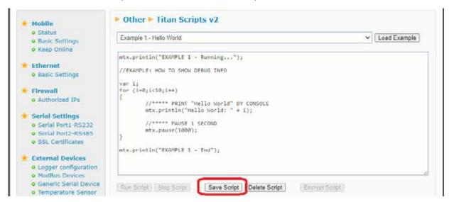
You can see that the example is very simple. It basically displays the text "Hello Word: X" 10 times. The debug console is the window immediately below the code window. This window very useful for debugging scripts. All Strings passed to the "mtx.println()" function will be displayed on that screen.
