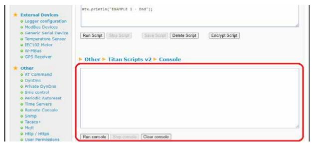
To run the script manually, just click on the "Run Script" button. The script will then be executed and the result displayed in the Console window, i.e. the "Hello World" messages sent using the "mtx.println()" function in the script.
