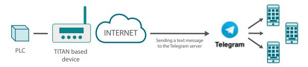
In this example, the address of the Modbus register to be read from the PLC will have Modbus address 0x01, and the Modbus read command used will be 0x03. Communication will be done using COM2 (RS485) of the Webdyn EasyTunnel, configured as 9600,8,N,1.
