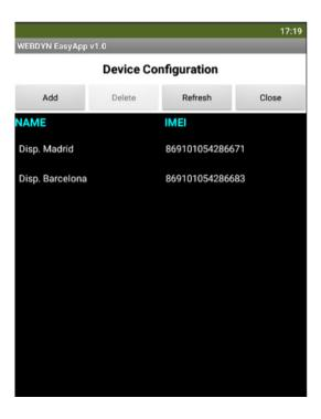
Now, press the "Select" button to choose the device you wish to communicate with. After selecting the device, click on the "List" button and choose the "getdata" command. Finally, click on the "Send Command" button at the bottom of the screen.
