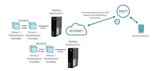
In this example scenario we will assume that Sensor 1 has the modbus RTU address @1 and Sensor 2 has the modbus RTU address @2. For both sensors, the modbus register for temperature will be the register with address "1", and for humidity the register with modbus address "2". RS485 port configuration is 9600,8,N,1
