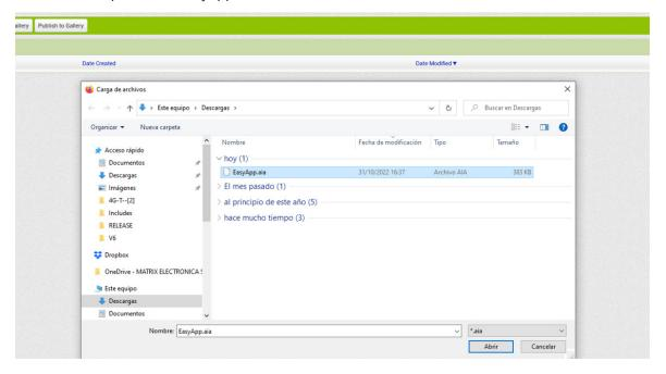
Once the project is loaded (we advise against modifying it this first time to check that everything works correctly), you can compile it from the menu "Build => Android App (.apk)", in order to generate the compiled file to install on an Android mobile phone.
