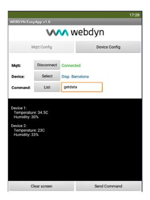
If, with the "List" button, we select the "custom" command, we can also specify AT commands such as the "AT+CSQ" command to obtain coverage, but it would also be possible to execute other AT commands remotely to read a digital input, to change or read the configuration, etc.
