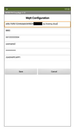
Once you have configured the MQTT broker configuration data, click on the "Save" button. If you then press the "Connect" button, the text "Connected" should be displayed in green, as shown in the image below. This will indicate that the APP has been successfully connected to the MQTT broker.
