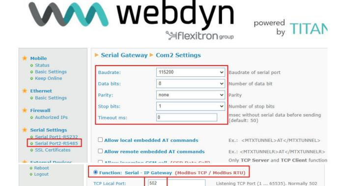
Once the TITAN-based device has been configured, we just need to Reboot and it will function as a Modbus TCP to Modbus RTU gateway.
