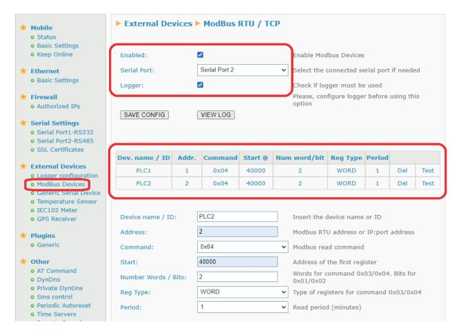
You will also enable the Modbus service by checking the "Enabled" box. You must select "Serial Port 2", since the reading will be made via the RS485 port. The "Logger" box must also be activated, since the Modbus registers read from the PLCs must be stored in the internal datalogger of the Webdyn EasyTunnel.
