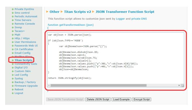
As indicated in the manual, this function to format the JSON is executed BEFORE storing the 1-read data in the internal datalogger and the JSON becomes a parameter with the standard format of the device, i.e. for example:
