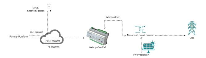
For this architecture to work, the WebdynSunPM gateway must have a permanent connection with the partner platform. This is possible either through a particular mobile phone operator that provides a public IP address and a VPN, or by installing the gateway behind a router in the photovoltaic power plant's information system.
