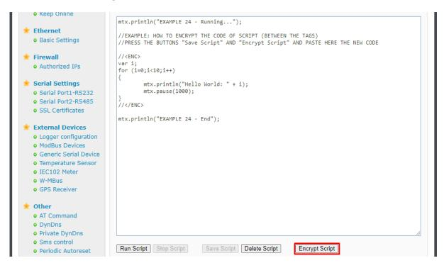
After pasting this new code into the script, the TITAN-based device will be able to run it in the same way.
