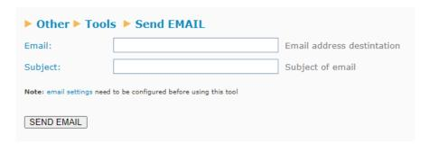
This feature allows you to check the correct configuration for sending emails from TITAN-based devices. To do this, the "Other→Email" section must first be configured.
