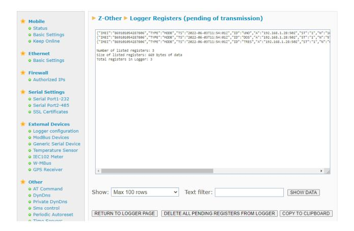
In this section, you can also delete all the data pending transmission by the TITAN-based device by clicking on the "DELETE ALL PENDING REGISTERS FROM LOGGER" button. You can also filter by text.
