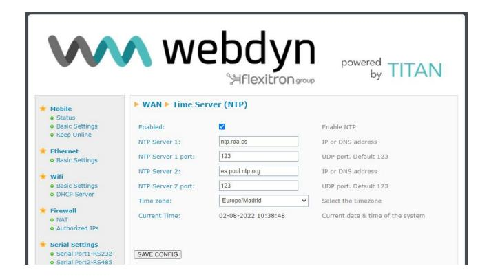
It is also possible to configure the Titan-based router as an NTP time server. To do this, simply check the "Enable" box and select the desired UDP port (by default, 123). It is useful, for example, to set the time correctly on devices even without using a SIM card (as long as it is a GPS-enabled Titan model).
