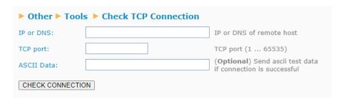
This feature allows you to check if a TCP port is available for connection from the point of view of the TITAN-based device. To check this connectivity, the device creates a TCP Client socket, which attempts to connect to the specified IP/DNS and TCP port. If the connection is made successfully, the result will be shown as successful. You also have the option to add an additional ASCII data field, which the TITAN-based device will send via this socket once the connection has been made.
