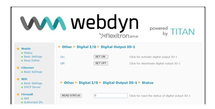
From this screen, it is possible to change the status of a digital output and read the current status of the output. Remember that it is also possible to change the status of a digital output from TITAN Scripts.
