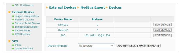
This table shows the name of the device and whether it has a Modbus RTU or Modbus TCP address. If you click on the "**EDIT DEVICE**" button of one of the devices, you will be directed to the editing screen for the corresponding Modbus registers of that device.
