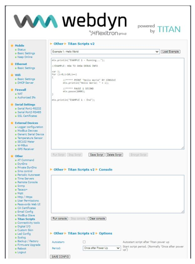
In the top drop-down menu, you have multiple examples of all the features you can use. To load an example, select the example of your choice from the drop-down menu (the "Hello World" example is recommended for the first time) and then click on the "Load Example" button. The source code of the example will then appear on the screen.
