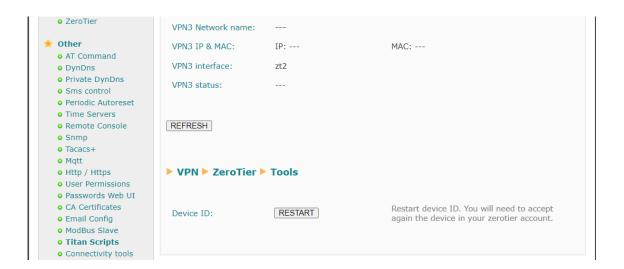
Restart: Button to change the Device ID of the ZeroTier network device. If the Device ID has been changed, you will need to go to the ZeroTier control panel (my.zerotier.com) and re-authorise the device on the network.
